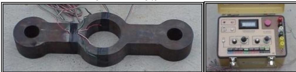
Figure 4 Circular ring type monolithic load cell and strain indicator.
