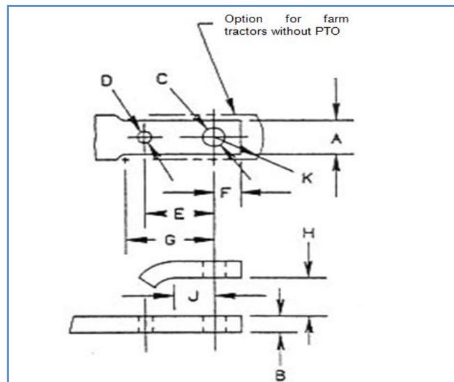
Figure 1 Drawbar tool of a farm tractor (Reprinted with permission from ASAE Standard S482 DEC98: Drawbars -- Agricultural wheel tractors. Copyright 1998 American Society of Agricultural Engineers. St. Joseph, Mich.: ASAE).
