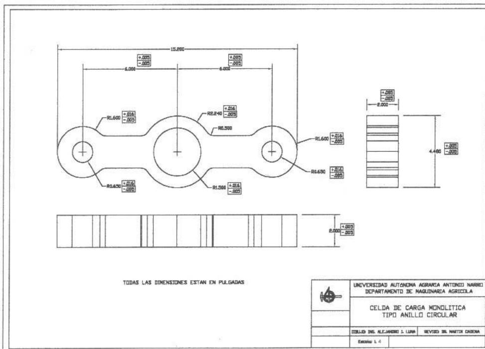
Figure 3 Circular ring type monolithic load cell.
