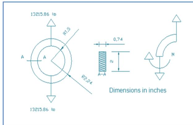
Figure 2 Stress analysis of load cell.
