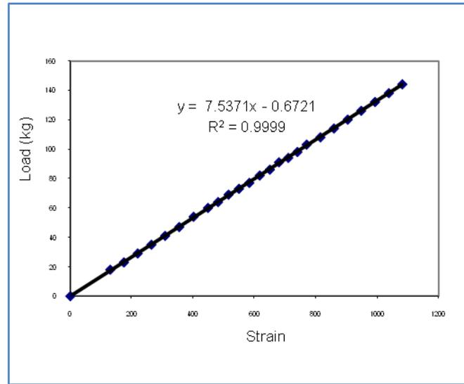
Figure 5 Calibration curve of a circular ring type monolithic load cell.
